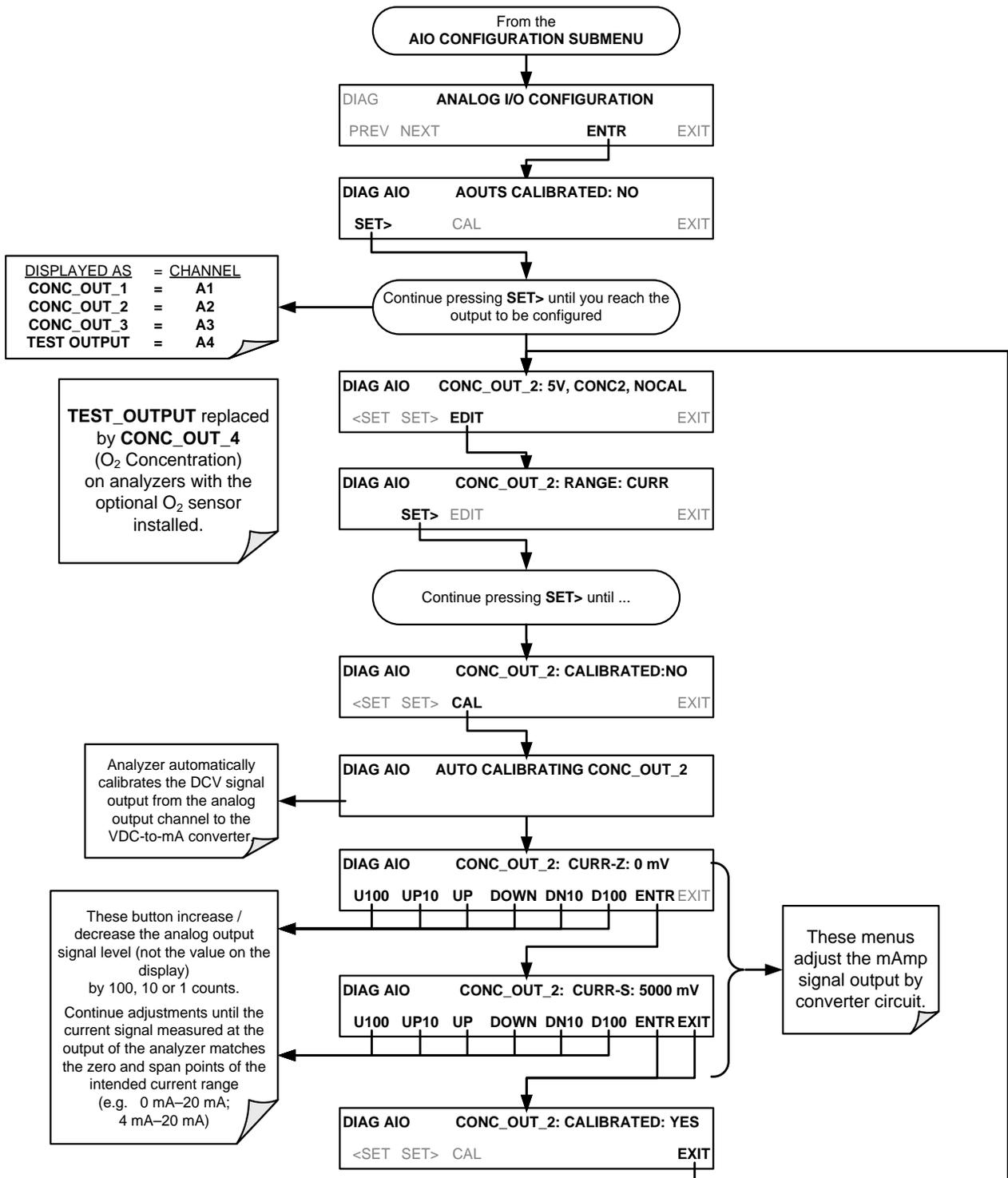
An alternate method for measuring the output of the Current Loop converter is to connect a 250 ohm  $\pm 1\%$  resistor across the current loop output in lieu of the current meter (see Figure 3-8 for pin assignments and diagram of the analog output connector). This allows the use of a voltmeter connected across the resistor to measure converter output as VDC or mVDC.
