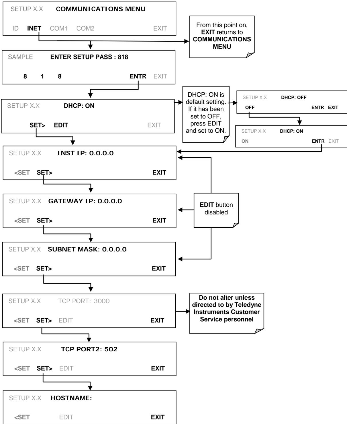
Figure 6-5. COM – LAN / Internet Automatic Configuration (DHCP)
