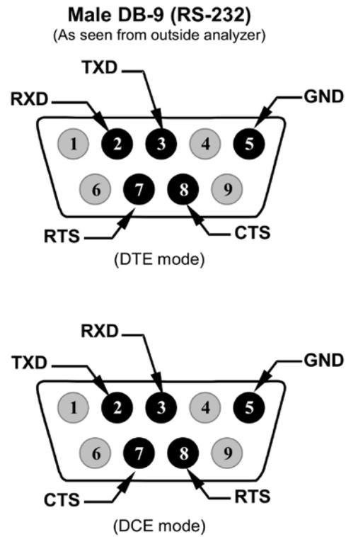
**Figure 3-13 Rear Panel Connector Pin-Outs for RS-232 Mode**
