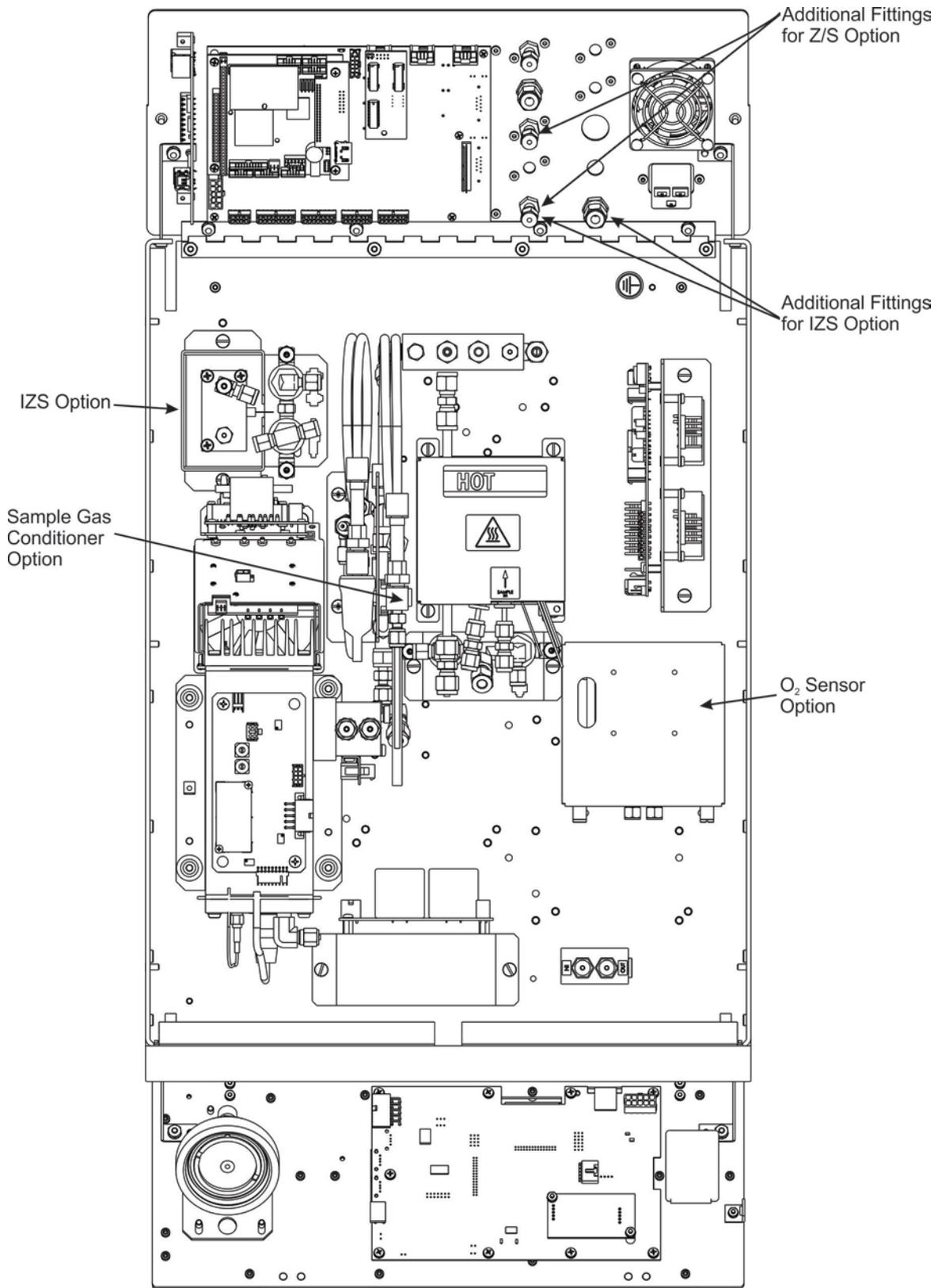
Figure 3-6: Internal Layout - Top View Showing Other Options
