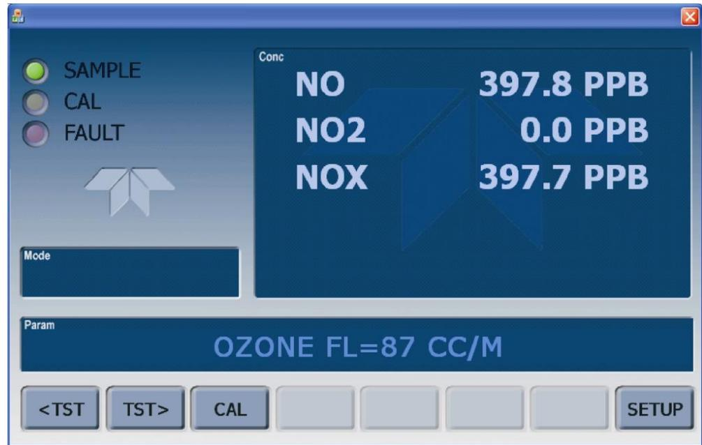
**Figure 3-2: Display Screen and Touch Control**
