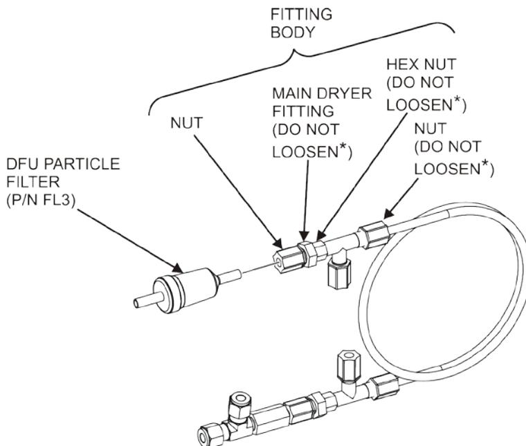
\* DO NOT LOOSEN THESE FITTINGS. HOWEVER, IF IT BECOMES NECESSARY TO RE-TIGHTEN THESE FITTINGS, ENSURE THAT THEY ARE TIGHTENED OVER THE PLASTIC INSERT AND THE O-RING OF THE INNER TUBING. TIGHTEN BY HAND AS MUCH AS POSSIBLE, AND THEN TIGHTEN 1/2 TURN WITH A WRENCH.
