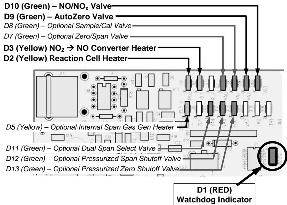
Figure 13-15: Status LED Locations – Relay PCA
