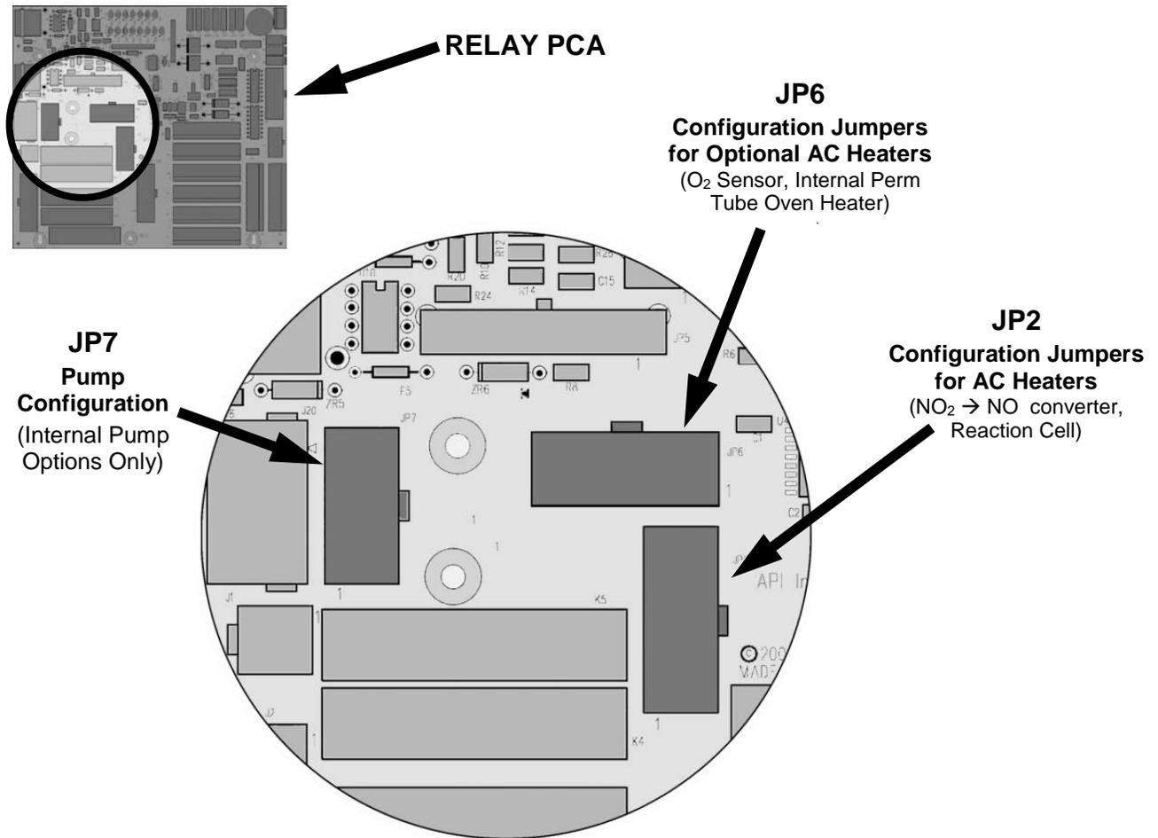
Figure 13-23: Location of AC power Configuration Jumpers
