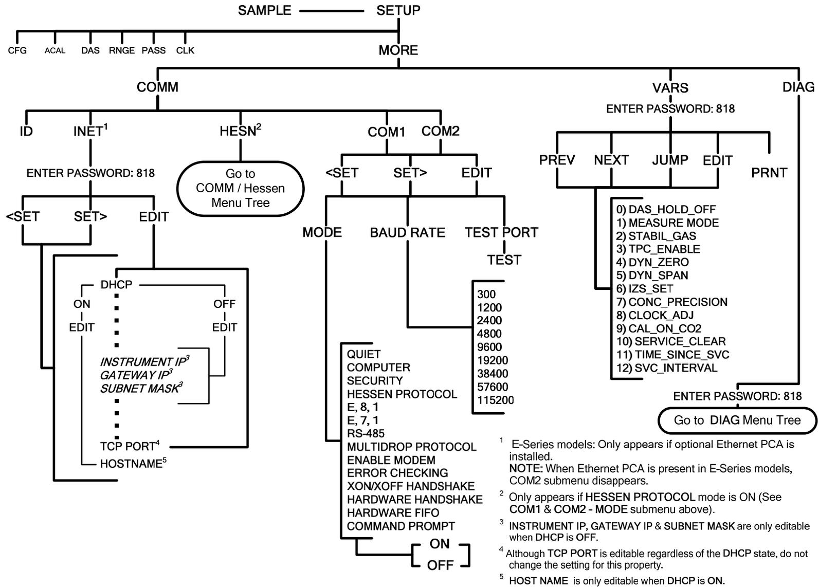
Figure A-3: Secondary Setup Menu (COMM & VARS)
