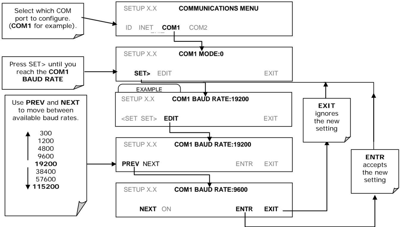
Figure 6-2. COM – COM Port Baud Rate
