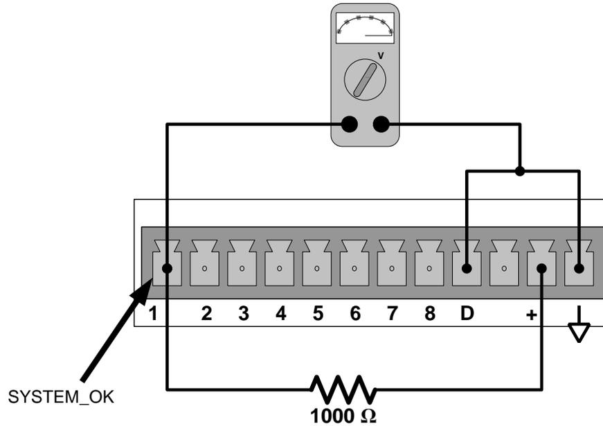
Figure 12-5: Typical Set Up of Status Output Test
