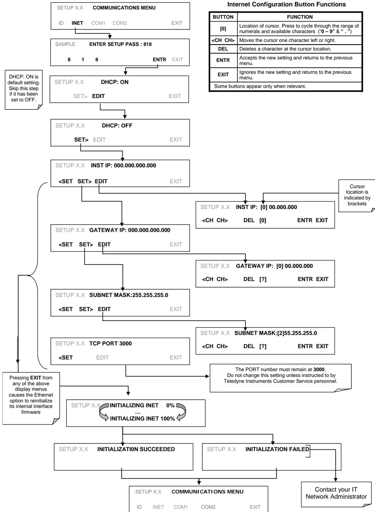
Figure 6-4. COM - LAN /Internet Manual Configuration
