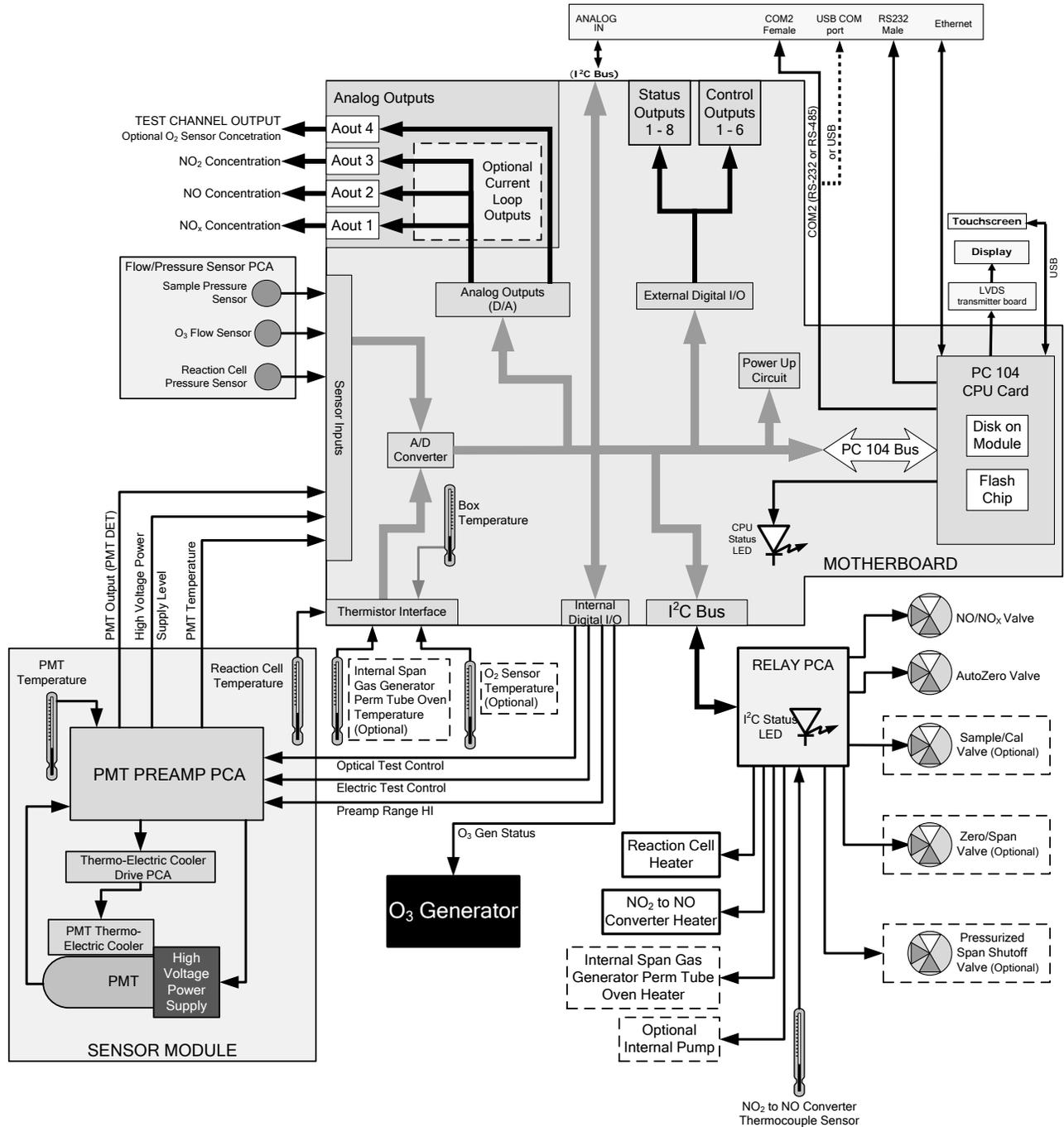
Figure 13-11: T200 Electronic Block Diagram
