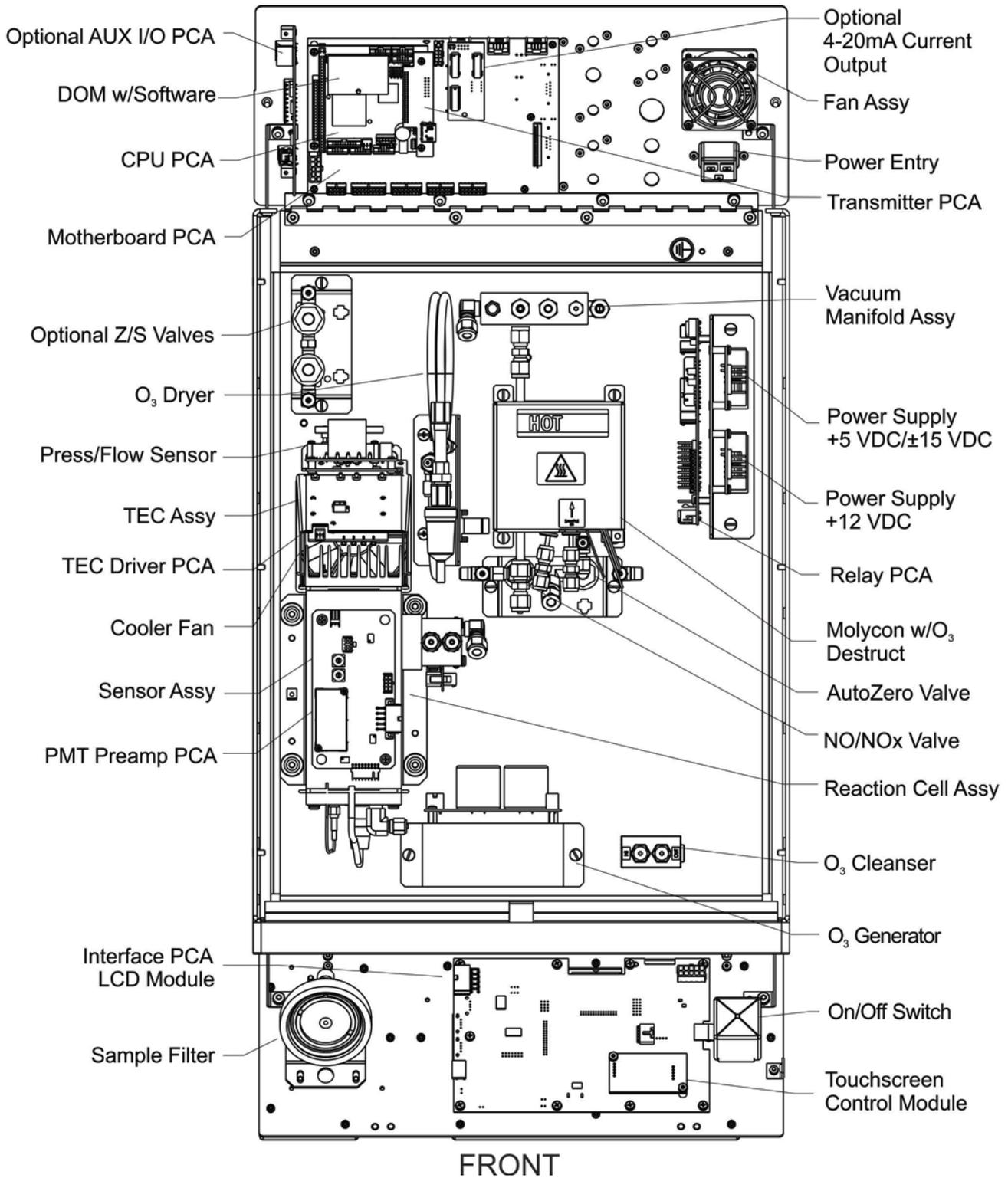
Figure 3-5: Internal Layout – Top View with IZS Option
