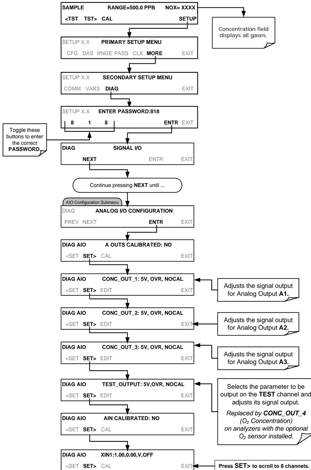
Figure 5-5: Accessing the Analog I/O Configuration Submenus
