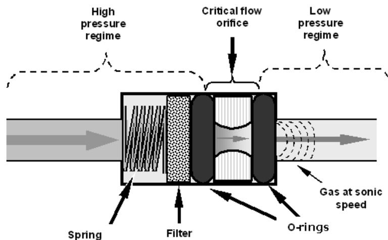
Figure 13-6: Flow Control Assembly &amp; Critical Flow Orifice
