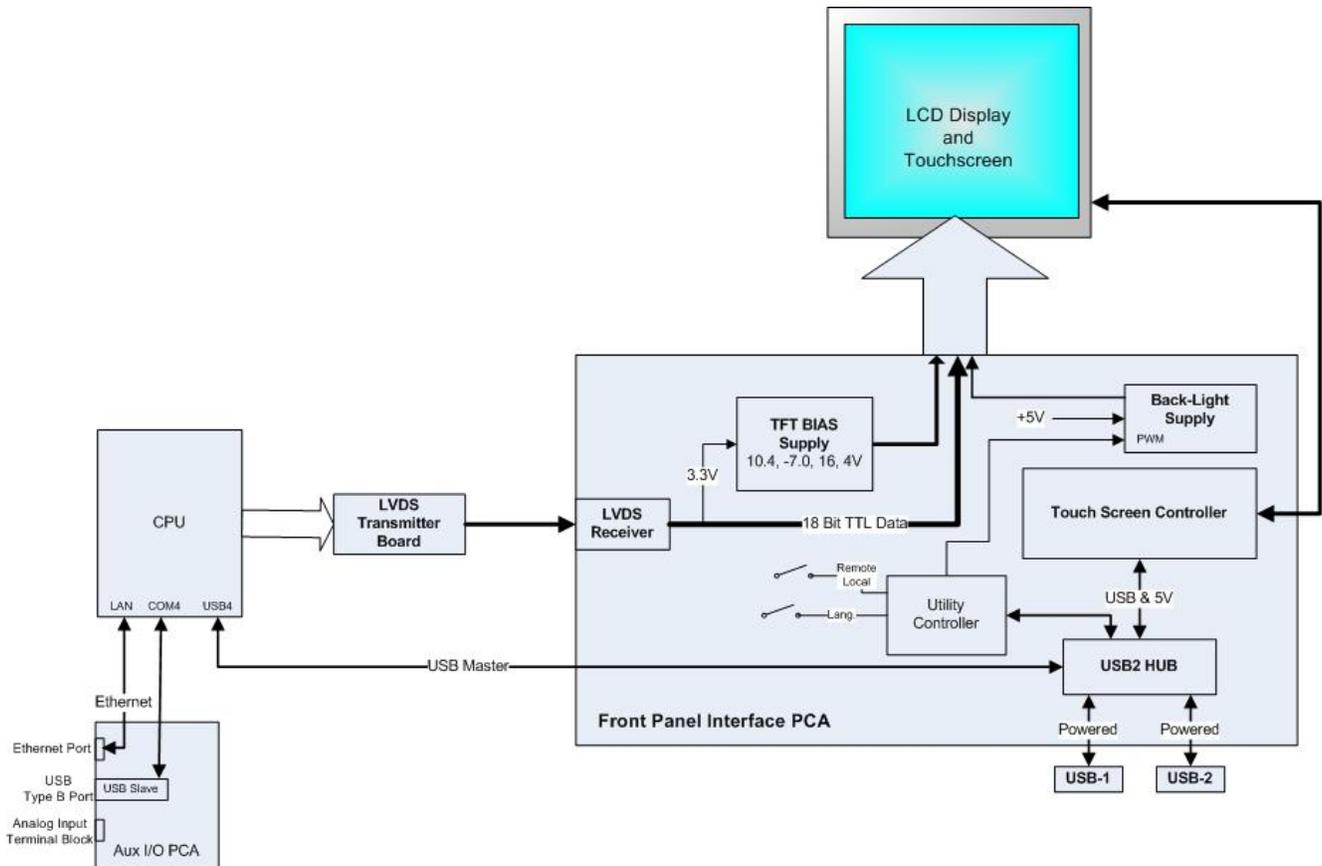
Figure 13-27: Front Panel and Display Interface Block Diagram
