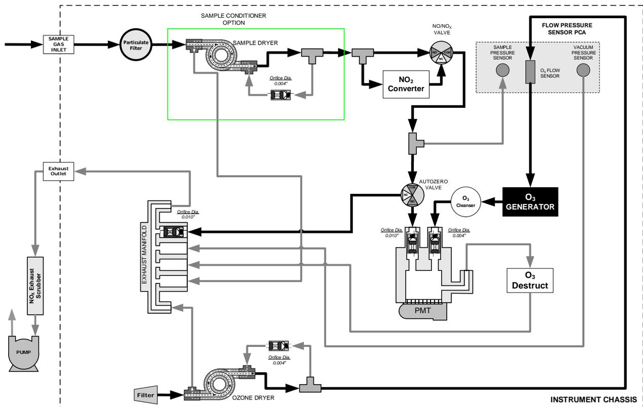
Figure 3-28: Pneumatics for Sample Conditioner OPT 86A
