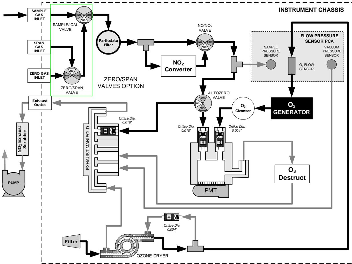
**Figure 3-22: Pneumatics with Zero/Span Valves OPT 50A**
