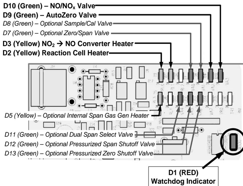
Figure 12-3: Relay PCA Status LEDS Used for Troubleshooting
