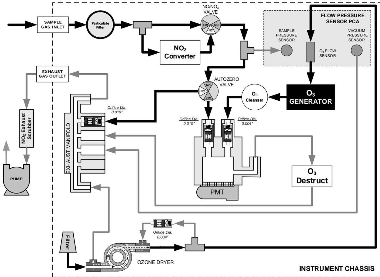
Figure 13-4: Pneumatic Flow During the Auto Zero Cycle
