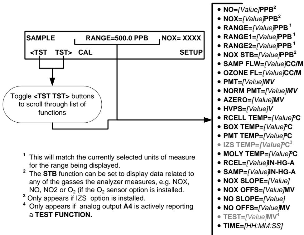
Figure 4-2: Viewing T200 Test Functions
