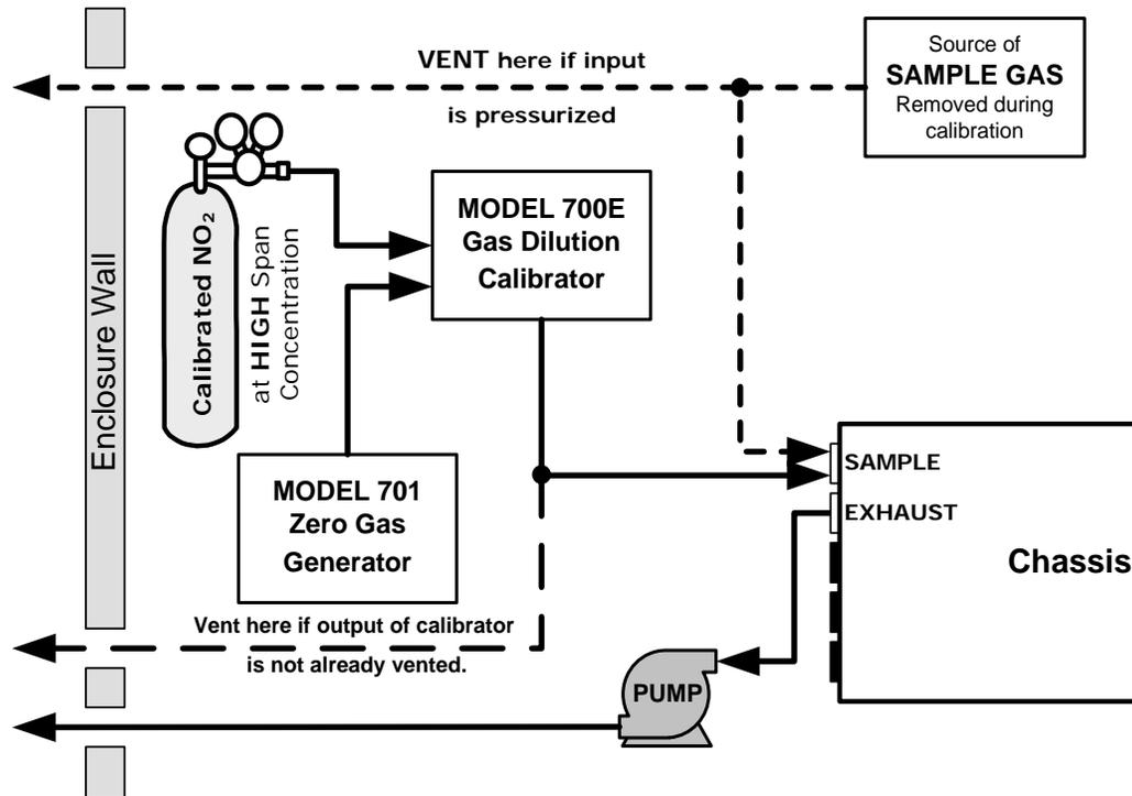
Figure 12-7: Setup for determining NO<sub>2</sub> → NO Efficiency – T200 Base Configuration
