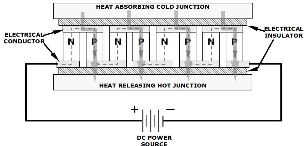
Figure 13-20: Typical Thermo-Electric Cooler
