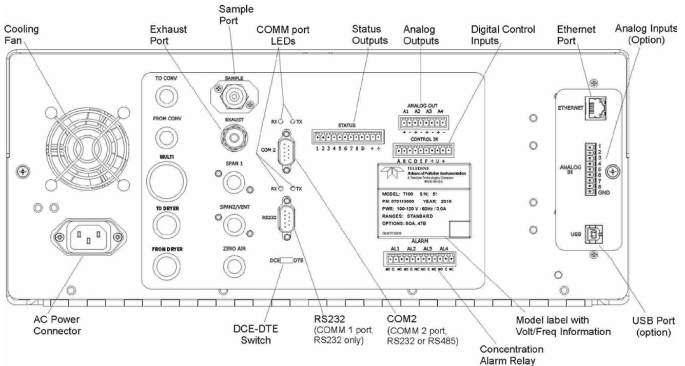
Figure 3-4: Rear Panel Layout – Base Unit
